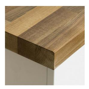
Then it's time to create our work surfaces from precisely manufactured solid wood blocks (staves) of seasoned timber. The staves are bonded together with finger joints and a specialist adhesive. The result? A beautifully strong surface with square cut ends that can either be retained for a contemporary feel, or machined to your own choice of profile. The decision, as ever, is yours.
