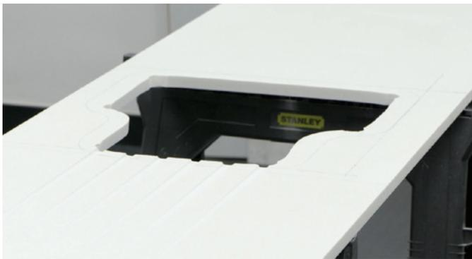
Once the adhesive has set, using a two-flute bottom bearing guide cutter, set the bearing so that it is contacting the uppermost inner face of the sink. Trim the excess material. Apply a rounded profile around the top edge of the sink. Finish the raw edge as described in the section 'Surface Finishing'.
