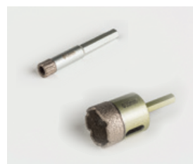
HOLE SAWS 12MM AND 35MM For starting hob or sink cut-outs and tap holes. (35mm should be used with Maxtop universal drill guide. Use MDF template for 12mm).
