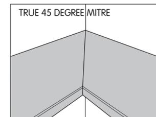
Care should be taken when trying to achieve a true 45 degree mitre as they can become weak at the narrowest point. Always ensure connector bolts are sufficiently used from the end point to prevent damage or breakage.
