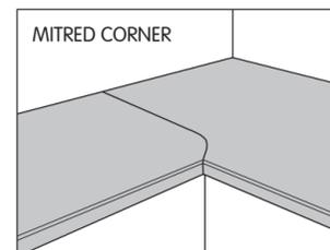
Jointing biscuits should also be used to add strength to the joint and ensure the joint is level. If in doubt consult a professional fitter.
