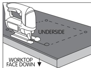
After drilling, turn the worktop over and mark a straight line from one edge of a hole to another. Then using a jig-saw with a fine toothed blade, cut from hole to hole. Ensure the piece to be cut away is well supported on the last cut. After the cut-out has been made, try the sink or hob for size.
