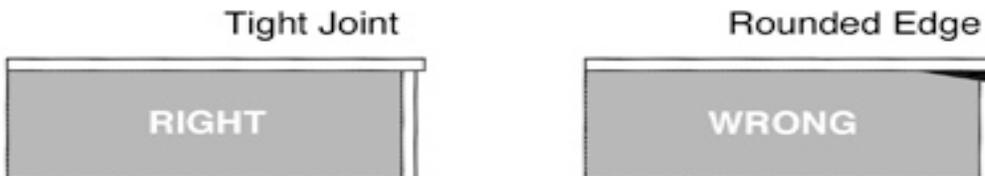
Machine the finished edge of the surface laminate with a bevel or radius cutter, and file or scrape smooth.
