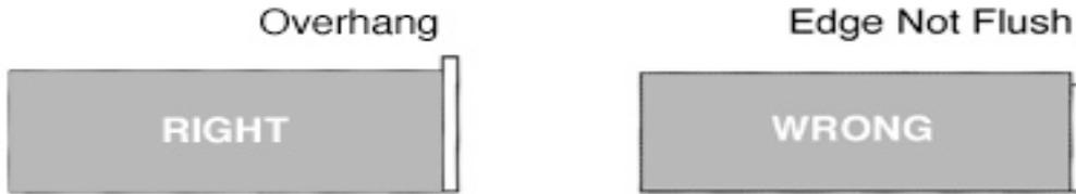
To avoid chipping, use sharp tools to machine Formica ColorCore flush with the substrate. When sanding, always work towards the substrate, using a fine grit sanding belt. Take care not to round-over the edge as this will result in a wide glue-line.
