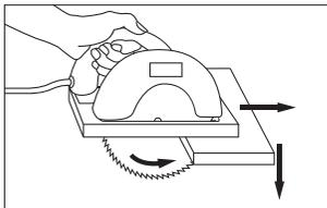
For best results when using an electric circular or jig saw, cut the Spectra Curved Edge surface face down so that the saw teeth cut into the laminate surface starting from the profiled front edge.
