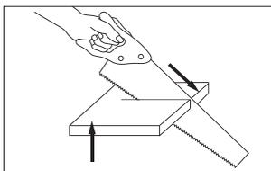
If using a hand saw, (10 to 12 teeth per 25mm) cut the Spectra Curved Edge surface face up. Always start from the profiled front edge and keep the saw at a low angle.
